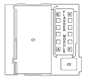
**<u>Fig. 34: Fuse Block - I/P Bottom View</u>** Courtesy of GENERAL MOTORS CORP.
