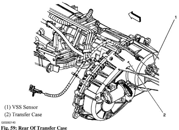
Fig. 59: Rear Of Transfer Case Courtesy of GENERAL MOTORS CORP.
