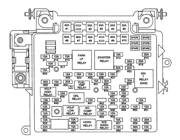
**Fig. 27: Underhood Fuse Block** Courtesy of GENERAL MOTORS CORP.
