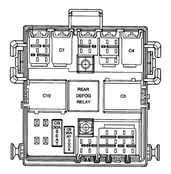
Fig. 30: Instrument Panel Relay Block Courtesy of GENERAL MOTORS CORP.
