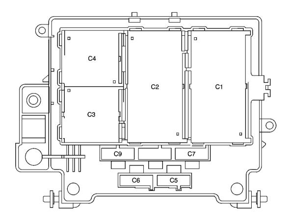
**Fig. 31: Fuse Block - Underhood Bottom View Courtesy of GENERAL MOTORS CORP.**
