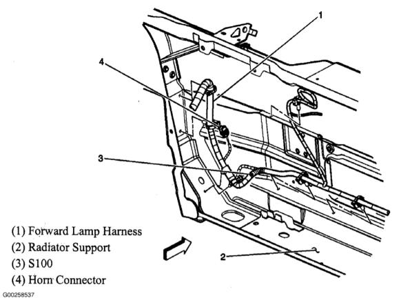
**Fig. 98: Left Front Of Engine Compartment Courtesy of GENERAL MOTORS CORP.**
