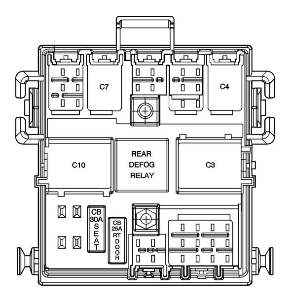
Fig. 36: Relay Block - I/P Top View Courtesy of GENERAL MOTORS CORP.
