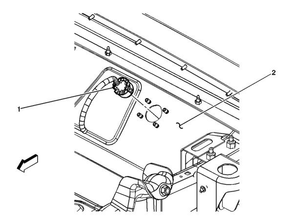
**Fig. 28: Trailer Receptacle Component Views Courtesy of GENERAL MOTORS CORP.**
