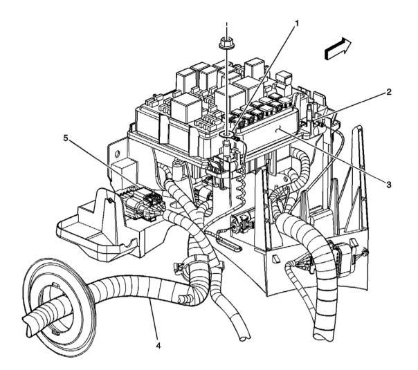
Fig. 1: Fuse Block - Underhood - Stud #1 and Stud #2 Component Views Courtesy of GENERAL MOTORS CORP.
