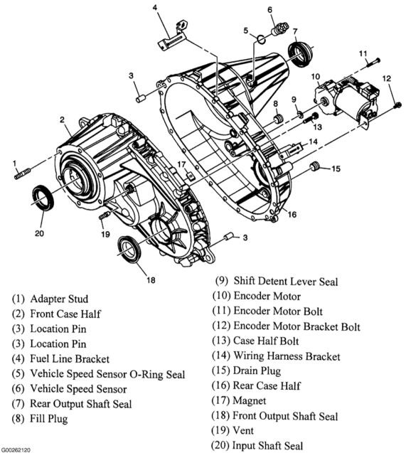
**<u>Fig. 41: Transfer Case</u>** Courtesy of GENERAL MOTORS CORP.
