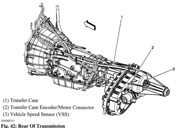
**Fig. 42: Rear Of Transmission** Courtesy of GENERAL MOTORS CORP.
