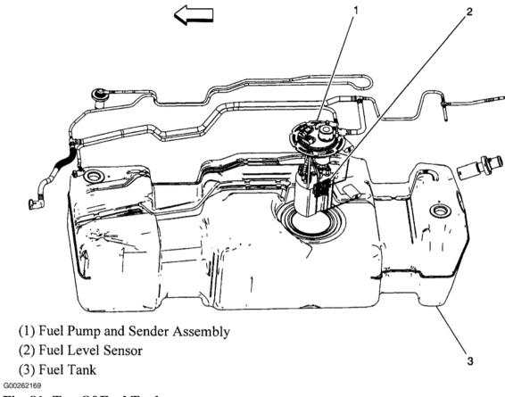
**Fig. 81: Top Of Fuel Tank** Courtesy of GENERAL MOTORS CORP.
