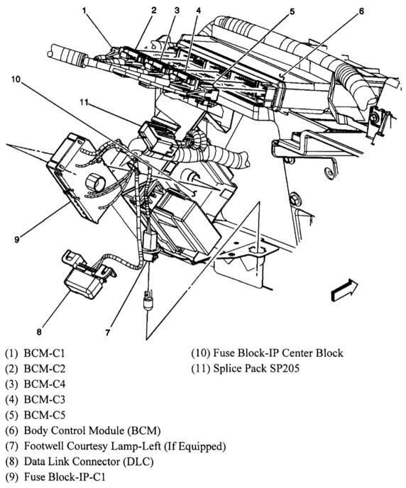
**Fig. 16: Left Side Of Dash** Courtesy of GENERAL MOTORS CORP.
