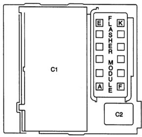
**Fig. 29: Bottom Of Instrument Panel Fuse Block Courtesy of GENERAL MOTORS CORP.**
