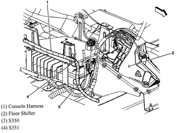
**<u>Fig. 89: Front Floor Console</u>** Courtesy of GENERAL MOTORS CORP.
