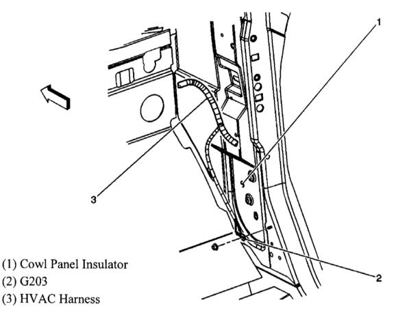
Fig. 15: Right Kick Panel Courtesy of GENERAL MOTORS CORP.
