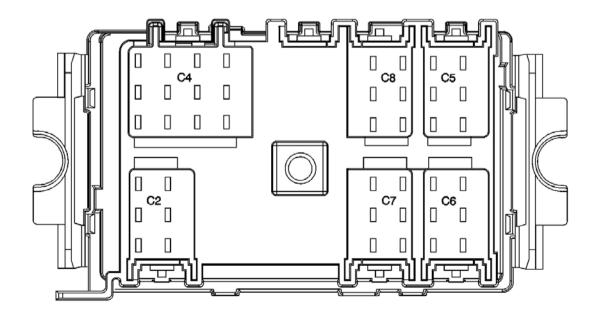
Fig. 38: Junction Block - I/P Top View
