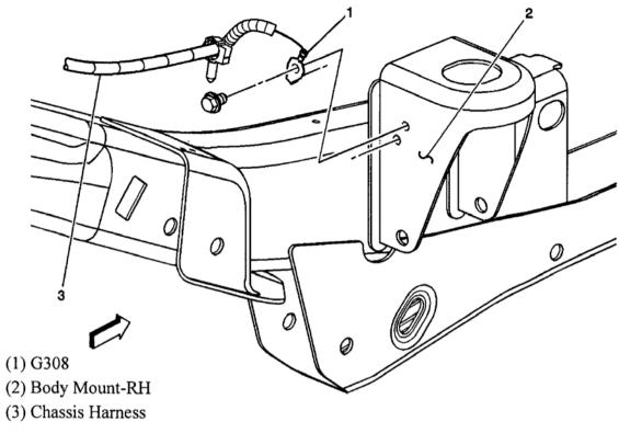
Fig. 21: Right Frame Rail Courtesy of GENERAL MOTORS CORP.
