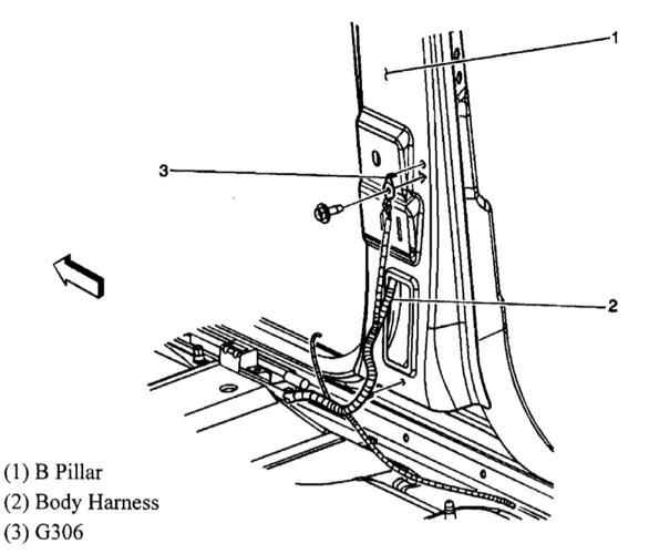
Fig. 20: Right "B" Pillar Courtesy of GENERAL MOTORS CORP.
